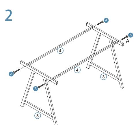
Attach 2 x frame [4] to 2 x frame [3] with 4 x bolt (A). Tighten with a screwdriver.
