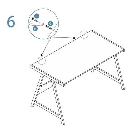
Move the unit to the desired location against a wall. Attach the other end of the 2 x safety straps (H) to the wall using 2 x wall plugs (G) and 2 x screws (F). Tighten with a screwdriver.
