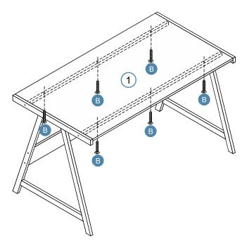
Attach panel [1] to the metal frame with 6 x bolt (B). Tighten with a screwdriver
